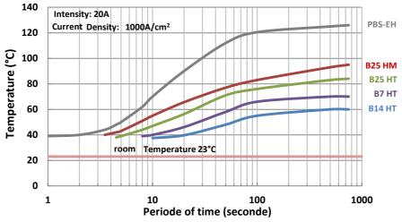
Heat resistance to a passing current of 20A and heat dissipation of copper-beryllium alloys. (Sample dimension :  $0,2 \times 10 \times 75$  mm)
