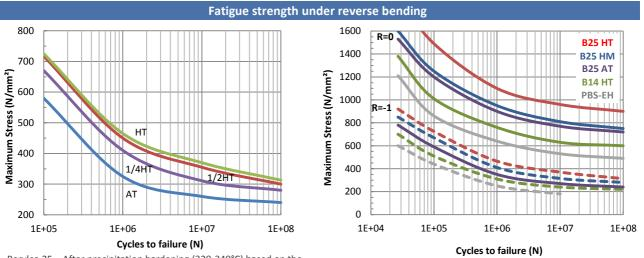
Berylco 25 – After precipitation hardening (320-340°C) based on the ASTM publication N°367
