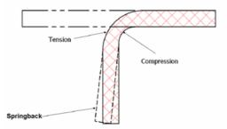
For a given thickness the amount of spring back increases with increasing yield strength and increasing bending radius. Therefore it is not unusual under normal manufacturing conditions to find variations in the same products when they originated from different manufacturing lots. When precise angular tolerances (less than 2°) must be maintained we recommend precipitation hardening in fixtures. See the chapter on 'Thermal Treatment'.
