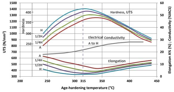
Properties of B25 and B33/25 alloys after age-hardening at various temperatures (retention time: 2 hours)
