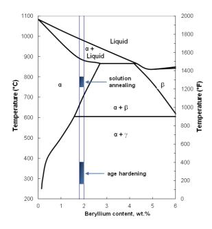
The solubility of beryllium in copper increases with increasing temperature, from practically zero at room temperature to more than 2% by weight at temperatures above 800°C. This zone is represented at the left of the diagram where the alloy is in solid solution (phase  $\alpha$ ), a face centred cubic structure like copper.
