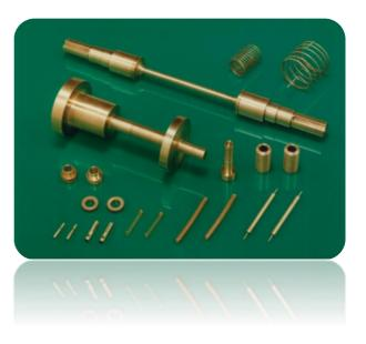
Alloy **Berylco 33/25** in any temper provides improved chip control due to a carefully controlled addition of lead. This alloy is well suited to automatic machining operations as the lead in the alloy reduces tool wear, eliminates clogging chips and produced small and short chips.
