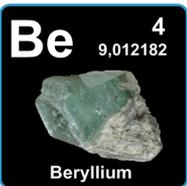
Beryllium (Be) is a mineral extracted from the ground mainly in an oxide state. A bivalent element, beryllium is a steel grey metal that can be mostly found in the minerals, the most important of which are beryl ( $\text{Be}_3\text{Al}_2\text{Si}_6\text{O}_{18}$ ), also called emerald and aquamarine according to its color, and chrysoberyl ( $\text{Al}_2\text{BeO}_4$ ). Pure beryllium is obtained by reduction of beryl or by electrolysis of beryllium chloride.
