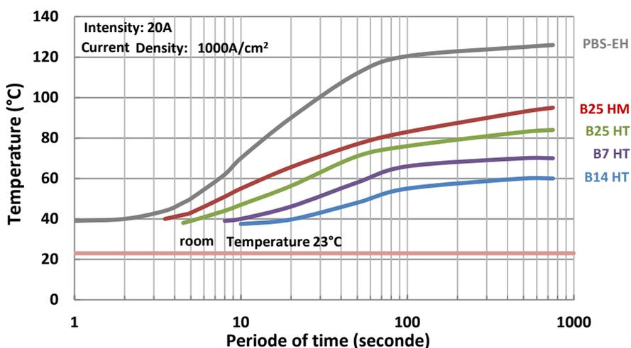
Heat resistance to a passing current of 20A and heat dissipation of copper-beryllium alloys.
