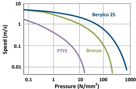
With lubrication, the friction coefficient of beryllium copper is significantly reduced (0.02 - 0.06) and wear resistance remains low even under high stress (500
