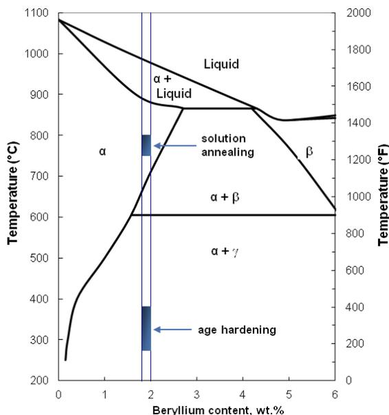
The solubility of beryllium in copper increases with increasing temperature, from practically zero at room temperature to more than 2% by weight at temperatures above 800°C. This zone is represented at the left of the diagram where the alloy is in solid solution (phase  $\alpha$ ), a face centred cubic structure like copper.
