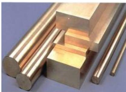
Rod and bar range on their cold drawn or extruded shape is extensive. Tubes are available in a wide range of diameter/wall thickness combinations such as ultra-thin tube walls to large size forged tubes. Tubes and bars can be delivered to the age-hardened condition. Rod, bar and tubes are primarily found in the annealed (A) and precipitation hardened (AT), as well as cold drawn (H) and precipitation hardened (HT).
